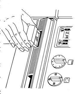
Insert the Vapour Guard, if required, into position at the top of the oven drawer.
