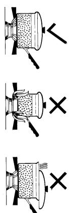
Bring items to the boil on the large flame setting then turn to the small flame setting for simmering. For maximum efficiency the flame should always remain underneath the pan and in order to save time and energy always try to cook in a pan with a lid on. Do not use an asbestos mat or anything else under the pan to spread the heat as this will cause damage to the burners.
