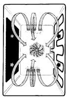
2. Fan Assisted [A] – the fan oven operates by constantly moving heated air around the oven. This gives improved efficiency and, in general, enables the use of lower temperatures for cooking. It also means that there is less need to be particular about shelf positions and that you can bake at more than one level simultaneously.
