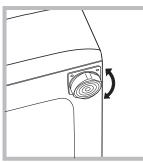
1. Install the washing machine on a flat sturdy floor, without resting it up against walls, furniture cabinets or other. 2. If the floor is not perfectly level, compensate for any unevenness by tightening or loosening the adjustable front feet (see figure); the angle of inclination, measured according to the worktop, must not exceed 2°.
