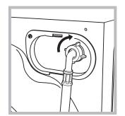
2. Connect the other end of the water inlet hose to the washing machine, screwing it onto the appliance's cold water inlet, situated on the top righthand side on the rear of the appliance (see figure).
